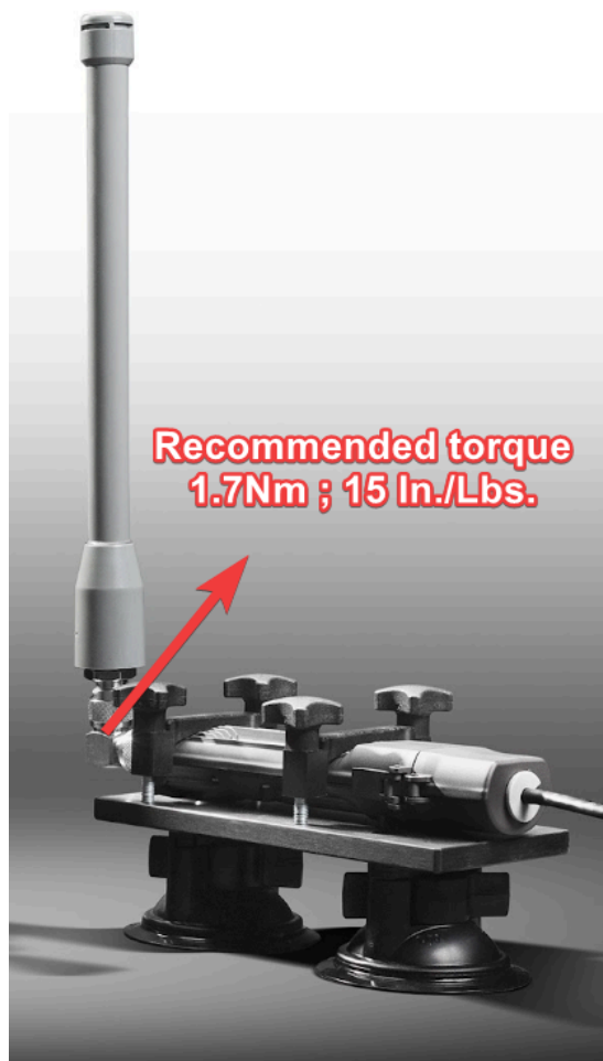
Image 1: Antenna mounting torque recommendation
