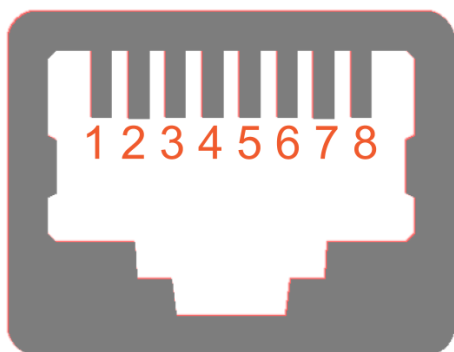
EtherCAT connector: pin-out (RJ-45 female)
