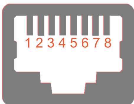
EtherCAT connector: pin-out (RJ-45 female)
