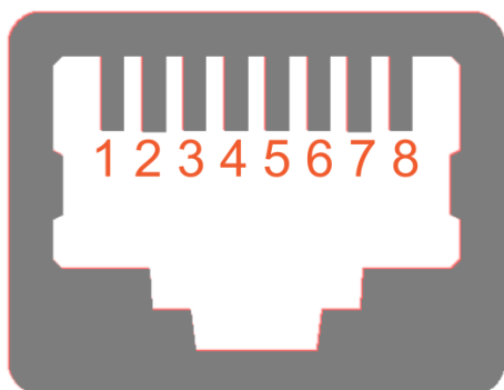
EtherCAT connector: pin-out (RJ-45 female)
