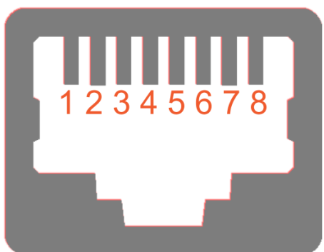
EtherCAT connector: pin-out (RJ-45 female)
