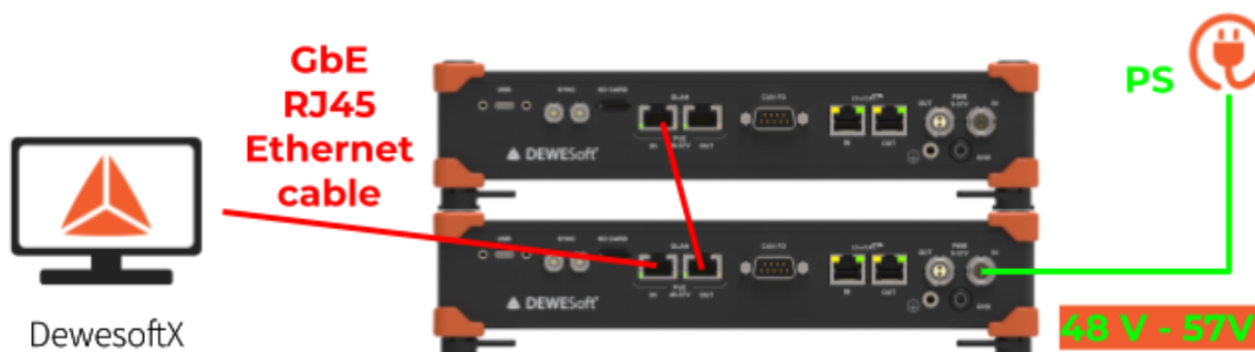
Connecting two SIRIUS X modules over EtherNET with PTP synchronization and with PoE connection
