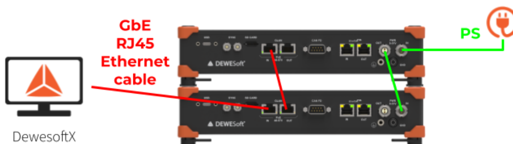
Connecting two SIRIUS X modules over EtherNET with PTP synchronization and without PoE connection
