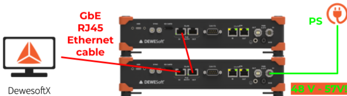
Connecting two SIRIUS X modules over EtherNET with PTP synchronization and with PoE connection
