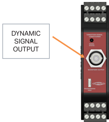
Figure 2. Signal Conditioner — Dynamic Signal Output BNC
