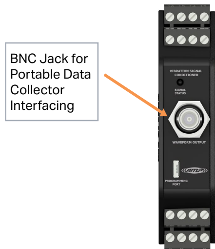
Figure 7. Signal Conditioner, BNC
